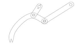
Figure 4: planting mechanism
